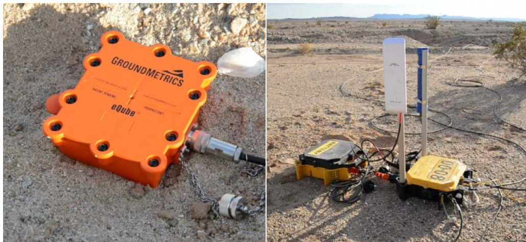
Figure 4. GMI sensing equipment. Left: Most recent GMI eQube sensor. Right: GMI data acquisition units.
